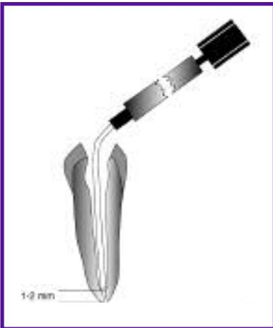
Using the root canal stop as your guide, place the needle into the root canal 1-2 mm from the apex. It should wedge in the apical portion of the canal. The needle can be bent for easy access, but do not crimp the needle.
